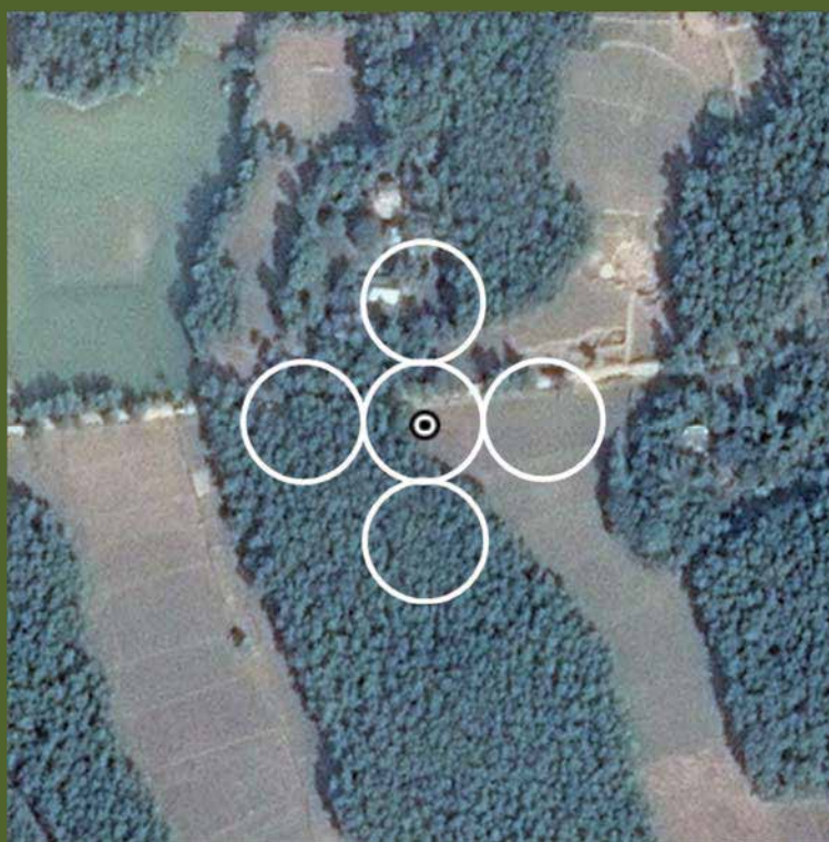
Figure 2.11: Accurate biophysical data collection depends on locating the plot center with high precision. The BFI uses DGPS technology to obtain cm level coordinates for future teams to navigate to the plot center.
