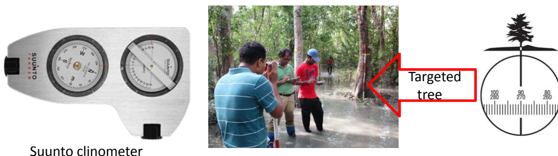
Figure 23: Bearing measurement using Suunto clinometer
