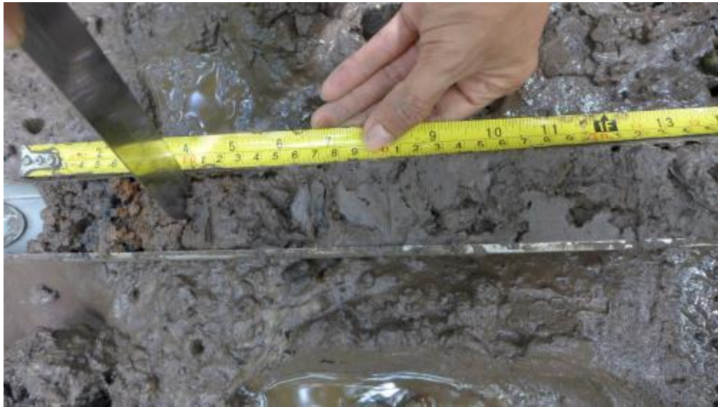
Figure3. Include the measuring tape when taking photos of soil samples (© Frida Sidik, FAO)
