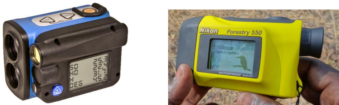
Figure 9. Vertex Laser (left) and Nikon Forestry (Right) range finders
