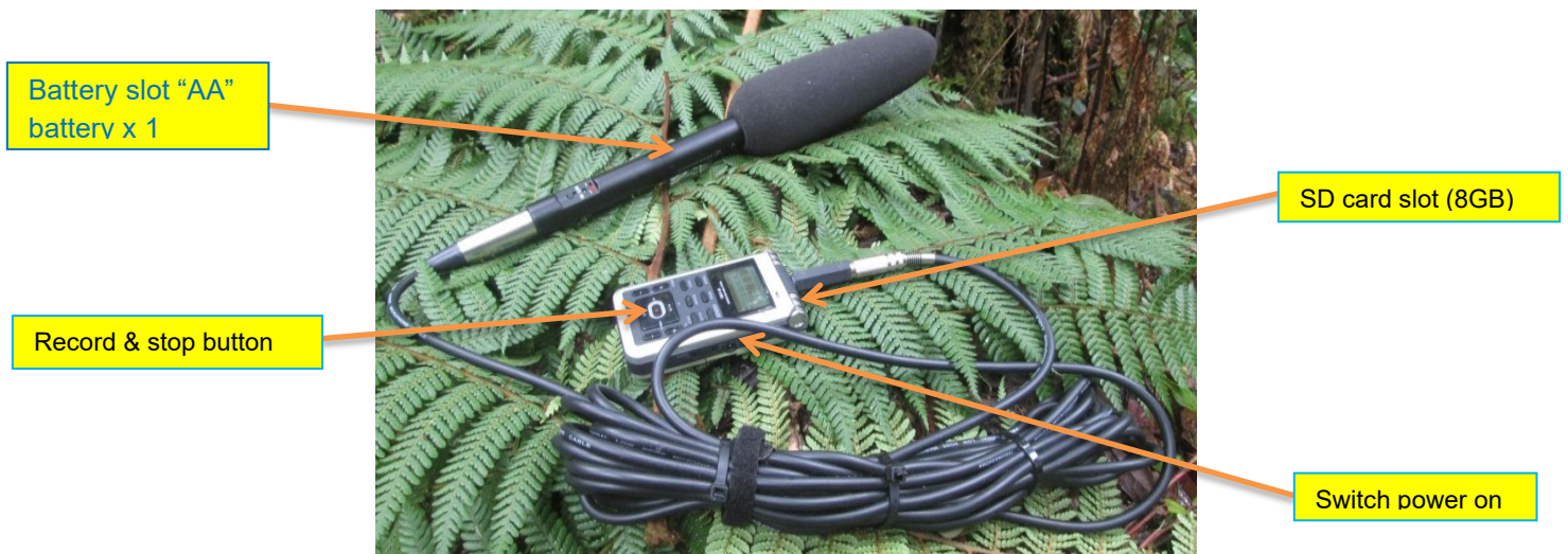
Fig. 2. The shot-gun recorder powered with two AA batteries inserted in the battery slot at the back of the recorder and one AA battery inserted in the battery slot of the microphone. One SD card (8GB) should be inserted in the card slot. Download all recordings using NFI laptops and transferred into two separate hard drives. Delete all files and re-use the same SD card at the next cluster. Repeat the same process/steps at the next cluster.
