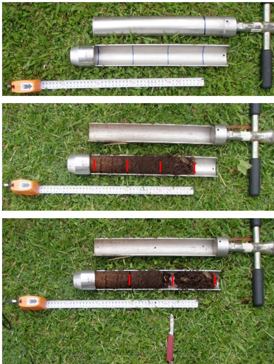
Figure 1. The Eijkelkamp sampler (A). This sampler is designed for topsoil sampling in stone-free soils. It is hammered into the soil to about 37 cm depth. The corer is then rotated to break the soil column and pulled out of the soil. One half of the cylinder is removed to reveal the 30+ cm core (B). This is cut into 10 cm lengths (measured from the top) for bagging as 0–10 cm, 10–20 cm and 20–30 cm samples (C). Cut and remove cores on a board or plastic sheet so that spilled soil can be retrieved.
